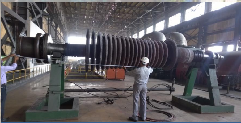
LP Stage of 95 MW unit being inspected for flaws
