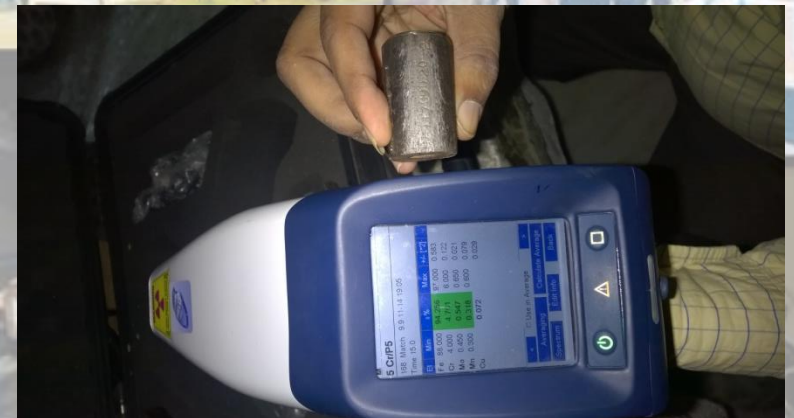
Positive Material Identification being done of Alloy Steel
