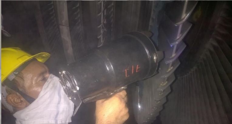
ITE's Engineer performing Fluorescent MPT of turbine blades
