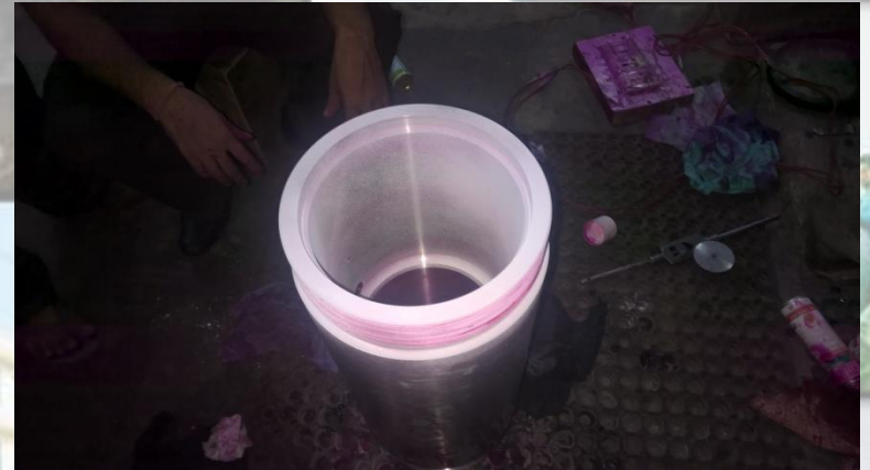
Visible Dye Penetrant Testing of Forged/Machined item
